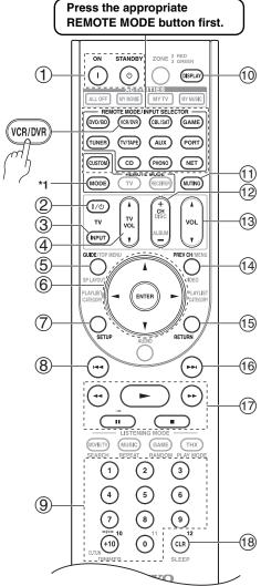
\*1 When you want to change the remote controller mode without changing the current input source, press the [MODE] button and within about eight seconds, press the REMOTE MODE button. Then, with the AV receiver's remote controller, you can control the component corresponding to the button you pressed.
